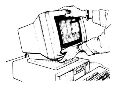
To produce an image that is clear and easy to look at, adjust the monitor's brightness and contrast controls. If your screen flickers, you can minimize it by selecting a dark background using either the brightness and contrast controls or your software.
